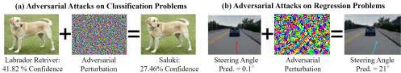
Fig. 2: Examples of adversarial attacks on image classification and regression tasks. Pixel values of perturbation \tau are scaled for visibility.
